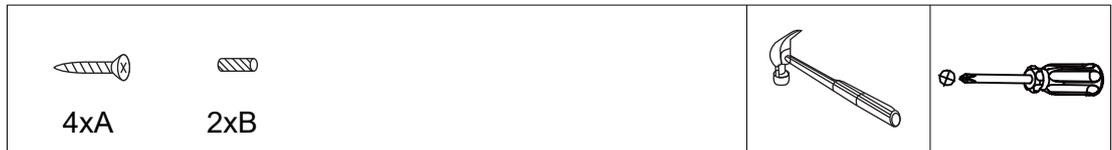
STEP 2: Fix panel (3) between side panel (1)&(2), using screw (A) and dowel (B).
