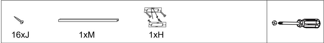
STEP 9: Join two back panels with filler (M), and attach back panel (11) to the body with screw (J).
