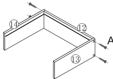
3A: Put bottom panel (15) into groove of panel (13)(14) and (12).
