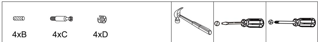
STEP 3: Attach panel (4) to panel (1)&(2), using dowel (B) and cam lock part (C)&(D).
