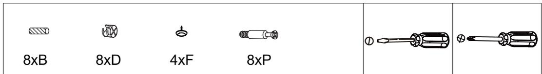
STEP 5A: Attach panel (6)&(7) to the body with dowel (B) and cam lock parts (D)&(P).
