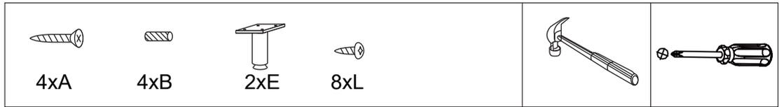
STEP 4A: Attach legs (E) to panel (5), using screws (L).
