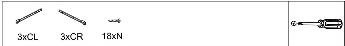
STEP 1: Install runner (CL) to panel (1)&(2) with screws (N) .
