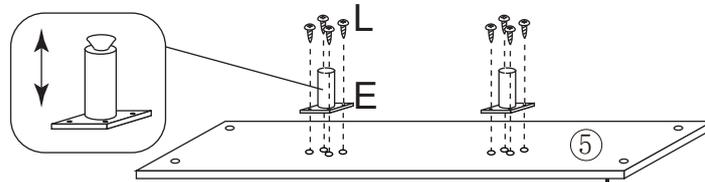
B: Attach panel (5) to the body with screw (A) and dowel (B).
