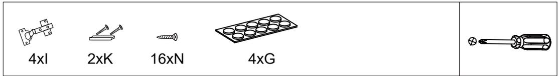
STEP 8A: Install hinges as shown in diagram, and stick part (G) to door corners to reduce noise when opening.
